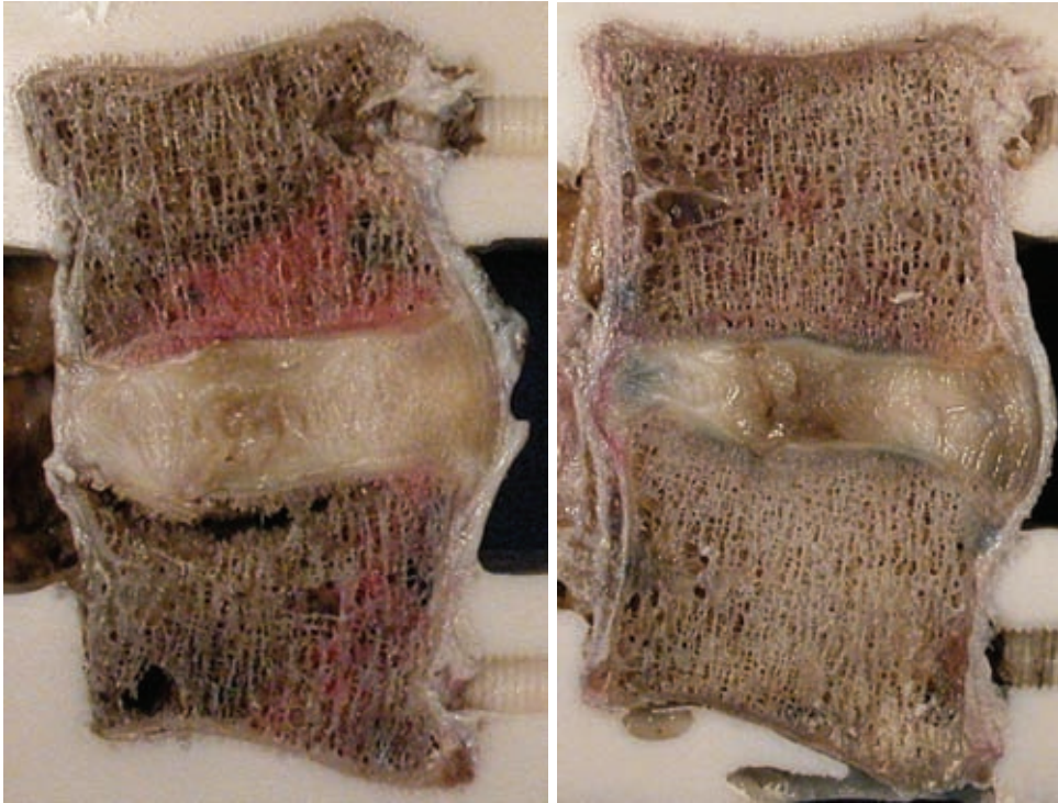
Figure II-25 Images of failed specimens tested in fatigue from the Old-Neutral group: LWS 1101 L4-L5 (grade 3.6) and LWS 1104 L4-L5 (grade 3.8), respectively
