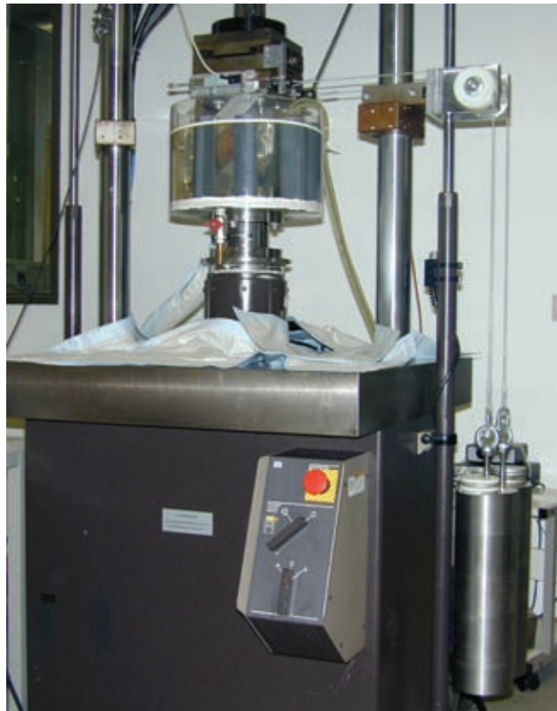
Figure III-5 Compressive pre-load is applied with dead weights connected to the upper attachment of the specimen with strings.
