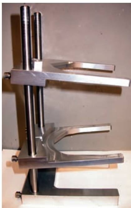
Figure II-3 Holder for potting and transporting the FSUs tested in flexed position
