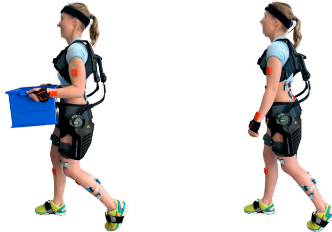
Figure 2. Tasks 2 and 3: carrying a box ( left ) and walking without load ( right ) with the exoskeleton PaexoBack.
